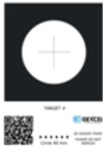
A circular target is a planar target printed as a white circle against a dark background. The value of internal diameter of the circle has not limitations.
